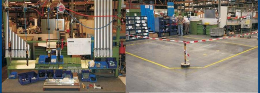
**Continually changing things one step at a time for the better ... that's KAIZEN. One improvement made by Siteco GmbH was to design a new manufacturing island for tunnel lights. Ergonomics and standards form the basis for introducing one piece flow. The goal is to eliminate inventory and to create the pull flow. It is a prerequisite that management promotes and supports continuous improvement and gives people opportunities to learn the skills and the time to practice them.**
